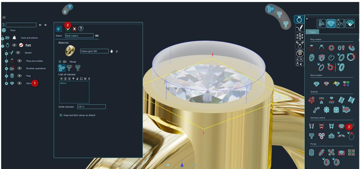
The drilling automatically adjusts to the size and position of the stone.
